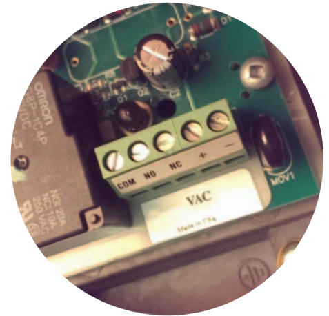
Figure R-7 DP-1C and DP-1D Terminal Block
