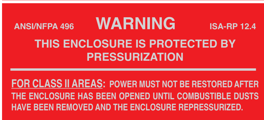
Figure F-9 Warning Labels to be installed on the enclosure in a readily visible location (Labels included in the AP-01 installation kit)
