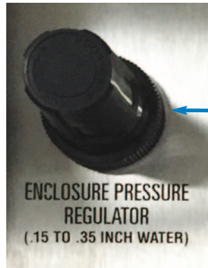
Figure F-12 Enclosure Pressure Regulator – Turn Counter Clockwise
