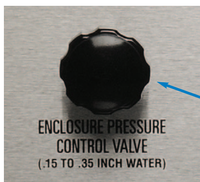
Figure F-10 Enclosure Pressure Control Valve
