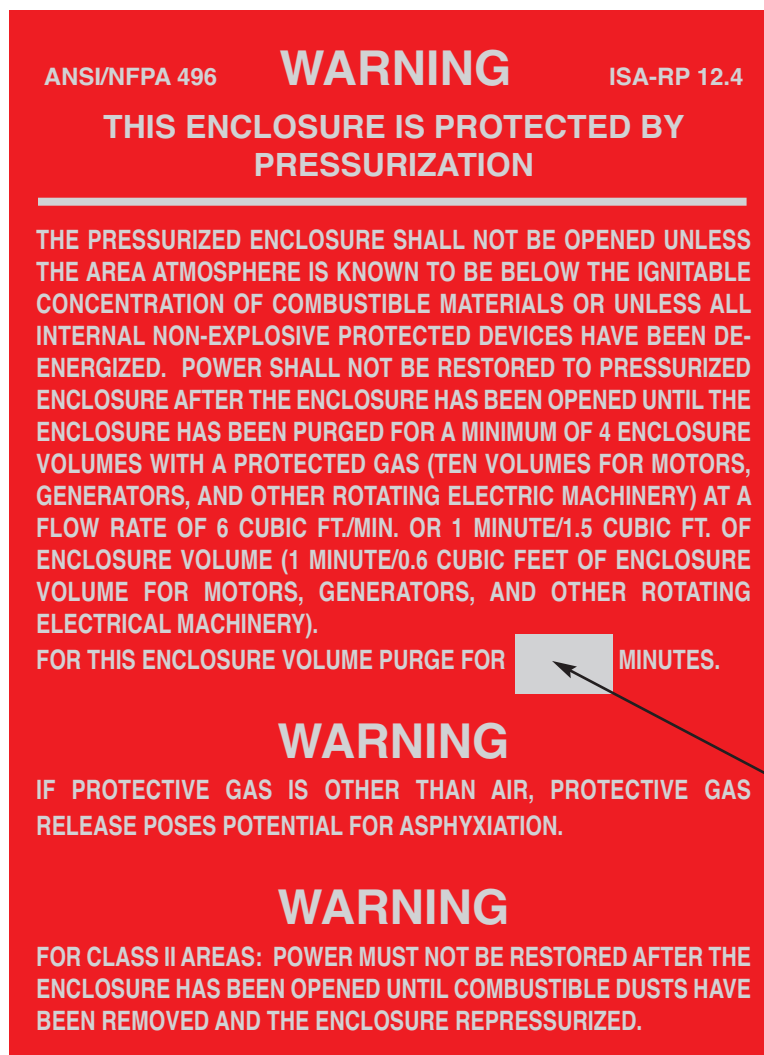
Figure F-1 Warning Label to be installed on the enclosure in a readily visible location (Label included in the AFP-01 installation kit)
