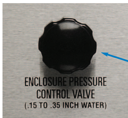
Figure F-10 Enclosure Pressure Control Valve
