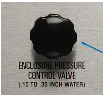
Figure F-16 Enclosure Pressure Control Valve
