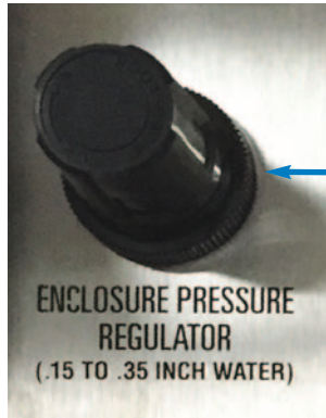
Figure F-13 Enclosure Pressure Regulator – Turn Clockwise
