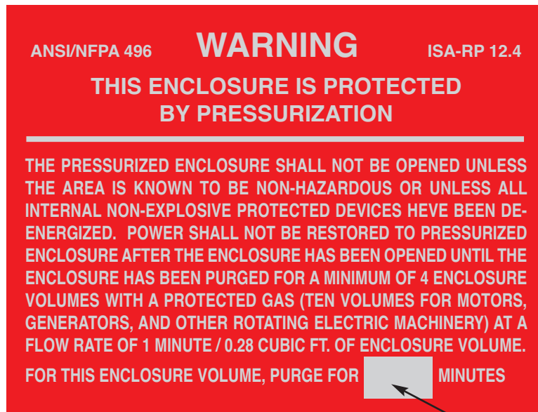
Figure F-1 Warning Label to be installed on the enclosure in a readily visible location (Label included in the AP-01 installation kit)
