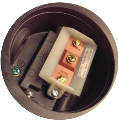
Figure R-5 DP-1A Terminal Block
